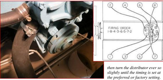
Don't forget to tighten down the distributor bolt. Keep in mind that Pontiac distributors rotate counterclockwise.
